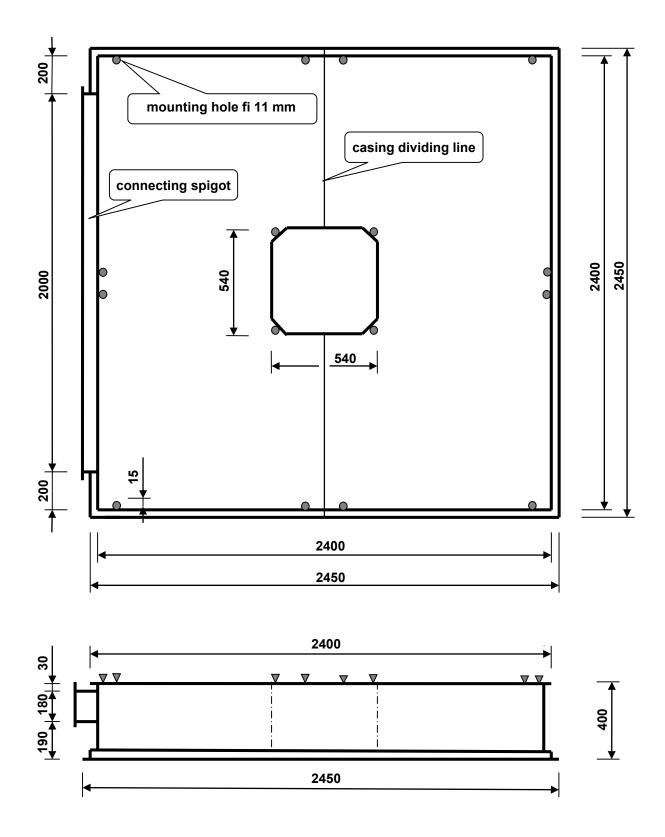
Fig. Example of the laminar ceiling LAM 2.4/2.4
